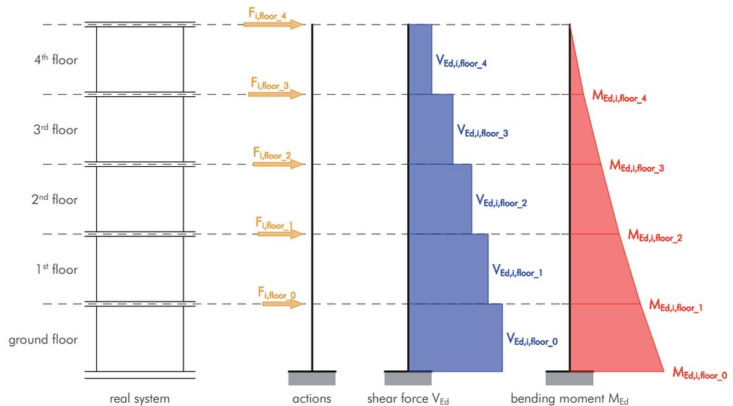
Fig. 4.2 cantilever-wall model with actions and internal forces
