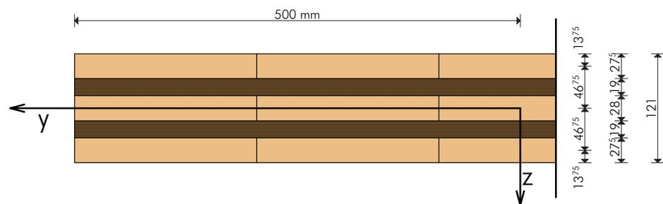
Fig. 3.4 cross section of the CLT panel
