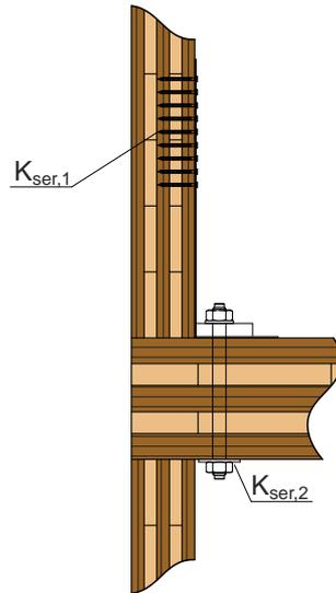
Fig. 2.4 wall-ceiling-wall connection joint with the hold down '480-M20' and the prevailing stiffness modulus
